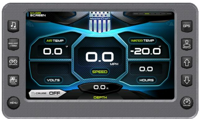
This screen shows the Speedometer, Air Temperature, Water Temperature, Battery Voltage, Water Depth and Engine Hours Gauges. The Cruise control can be turned ON or OFF from this screen by touching **[CRUISE]**.
