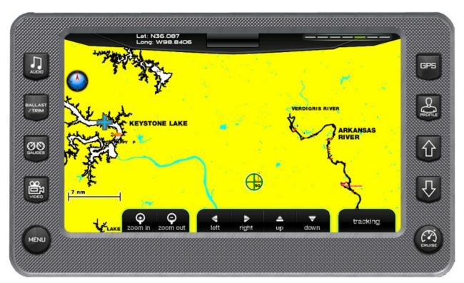
**UP – LEFT – RIGHT – DOWN ARROWS** – facilitates navigation of the GPS map by moving the
