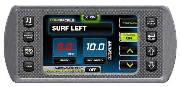
This feature displays rider/user profiles for cruise controls based on user preferences for speed, ballast, and smart plate settings.
